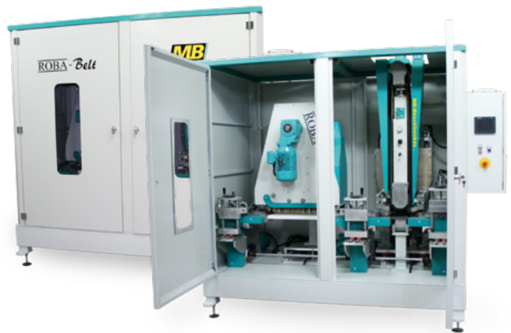
ROBA Belt configuration to process floor moldings using a BA300 belt sanding aggregate. The PLC activated and motor driven oscillation movement of all aggregates takes into account, beside the sanding belt grit, also the molding width. This ensures that the abrasives are always utilized completely.
