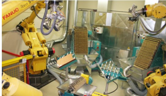
MB sanding machines integrated into a robot cell
