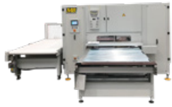
Machine with return conveyance for four sided edge sanding.
