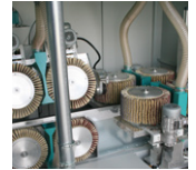
Fully automatic and all-round profile sanding
