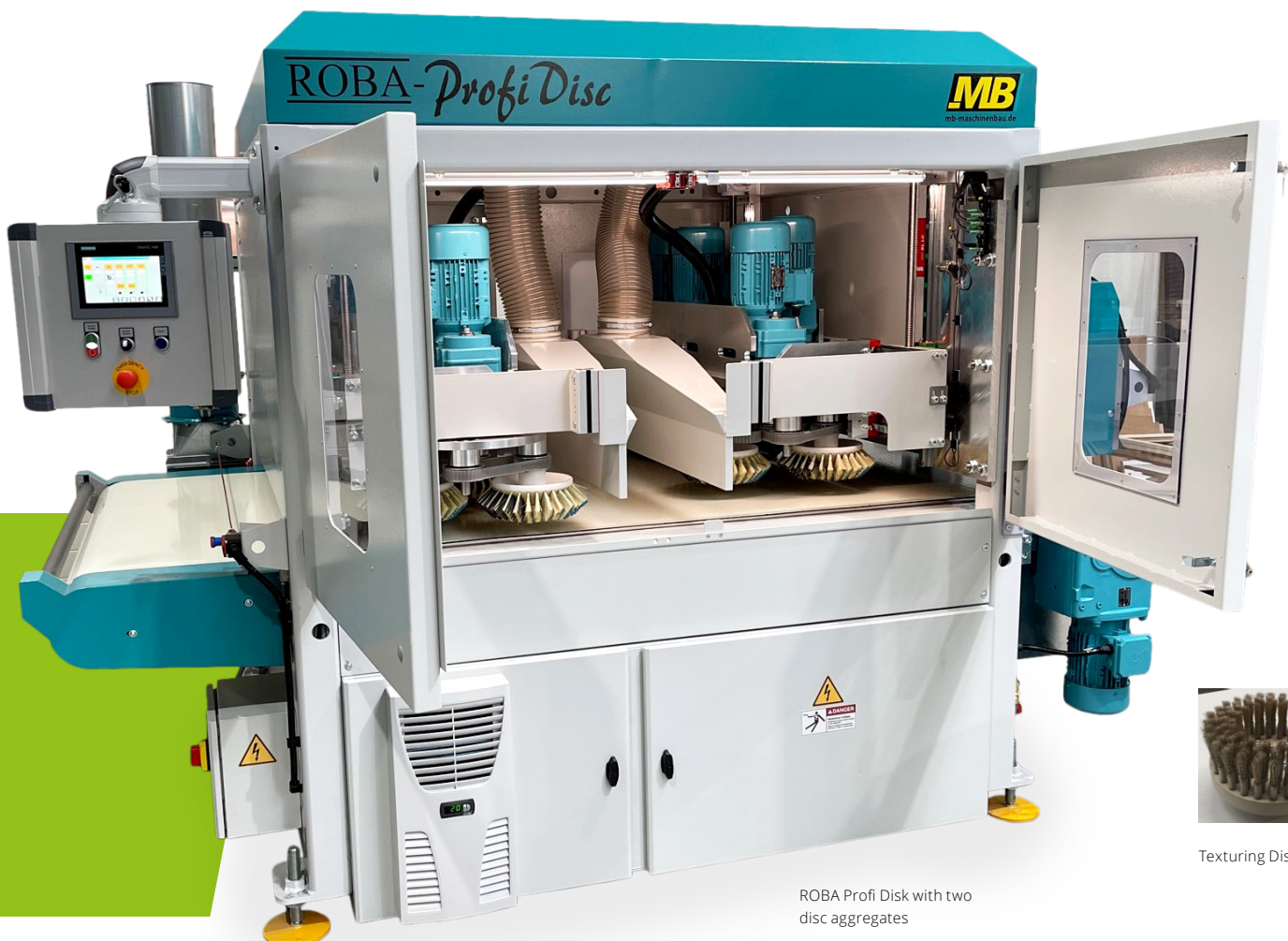
Micron Discs used to sand plane surfaces
