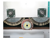
630 mm diameter: Comparison conventional (middle) – ROBA BIG (right and left)
