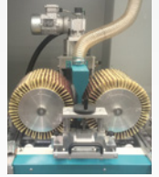
Double brush working clock- and counterclockwise
