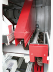
Transverse cleaning unit, optional also from bottom. On demand as brush or belt clean unit deliverable
