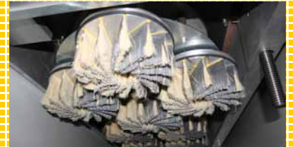
Profi Disc aggregate as an option at machine exit
