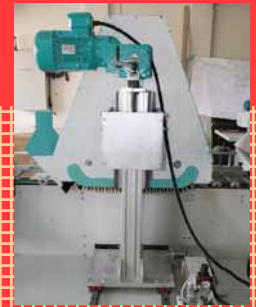
Rail guided oscillation and height setting at the column
