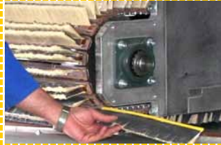
The sanding belt consists of easy interchangeable brush segments
